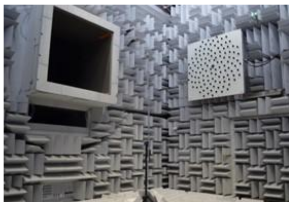
Figure 1: ISAE-SUPAERO SAA anechoic wind tunnel with the 120-channels microphone array used for aeroacoustic source localization.
