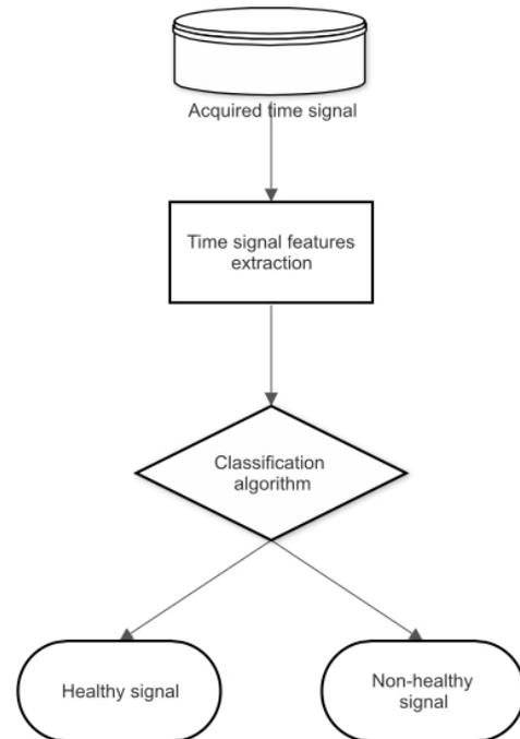
Figure 1. Flowchart for automatic time signal classification.
