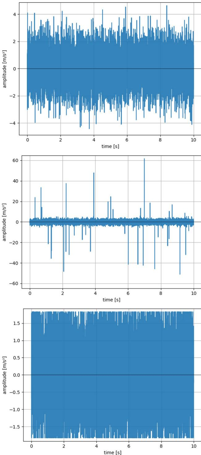
Figure 2. From top to bottom: stable signal (healthy), signal with impacts (non-healthy), signal with overload (non-healthy).
