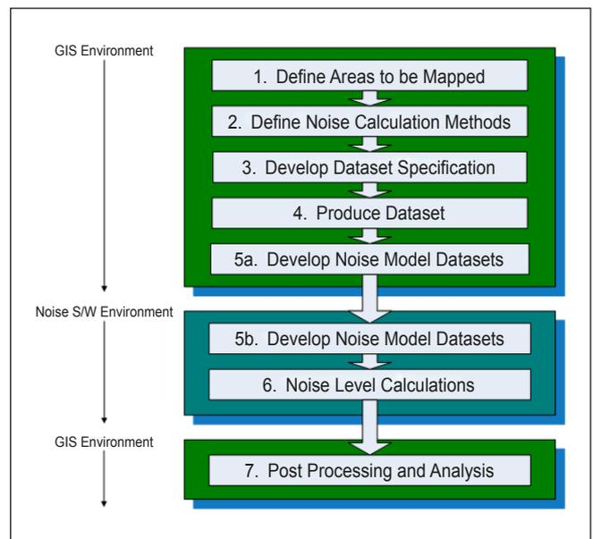
Figure 1. Overview of the noise mapping process [EPA Ireland [7]].
