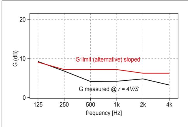
Figure 5.  $G$  values measured (@11.3 m) in final situation of 8,400 m<sup>3</sup> sport hall ( $T_{avg} = 1.3$  s) and allowed values (according eq. 1 and eq. 4).
