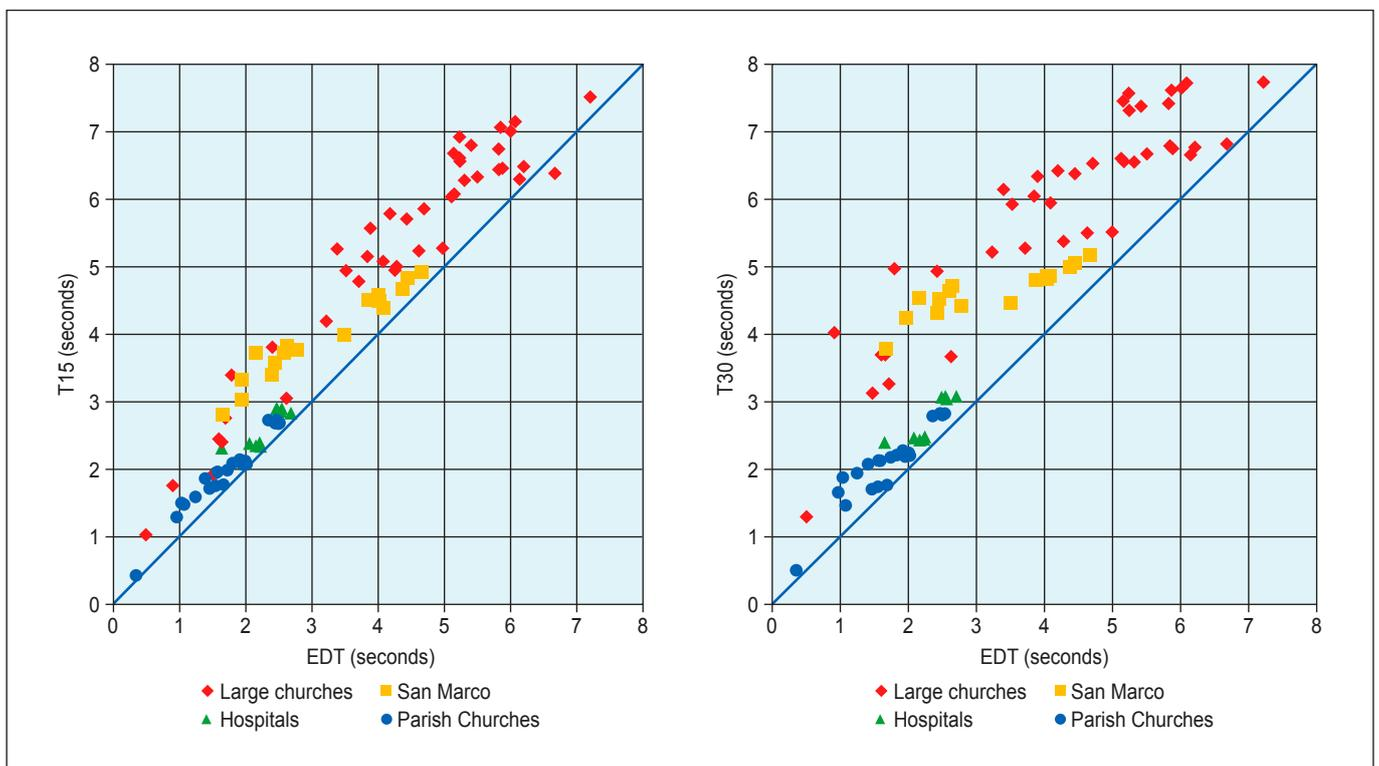
Figure 7. (a) A plot of T15 against EDT for all ten churches and all combinations of source and microphone positions for which data were taken. (b) The same plot as (a) for T30 against EDT for all ten churches. In both diagrams, a 45° line is shown.
