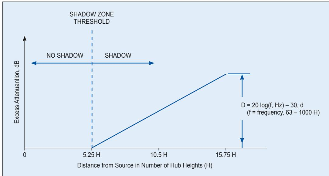
Figure 2. Upwind Noise Propagation from [7].
