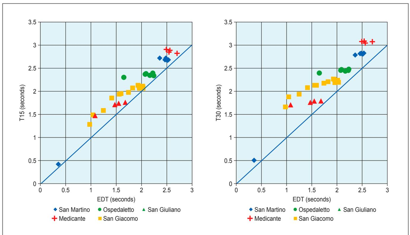
Figure 8. (a) A plot of T15 against EDT for five small churches and all combinations of source and microphone positions for which data were taken. (b) The same plot as (a) for T30 against EDT for the five small churches. In both diagrams, a 45° line is shown.
