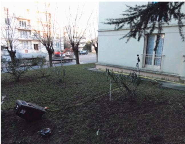
Figure 3. Example of façade sound insulation measurement in accordance with NF EN ISO 10052.
