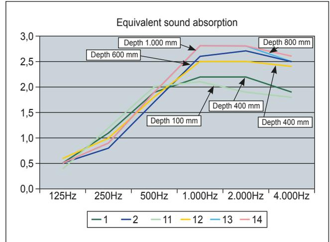
**Figure 8.** Examples of equivalent absorption area values per octave band, for glass wool free hanging horizontal units of 1.2 x 1.2 m suspended at 200, 400, 600, 800 and 1000 mm from the slab.
