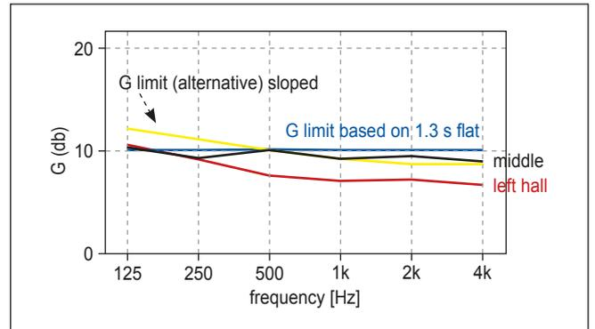
Figure 7.  $G$  values measured ( $r = 4V/S = 9m$ ) in 1/3 hall parts and allowed values (according eq.4).
