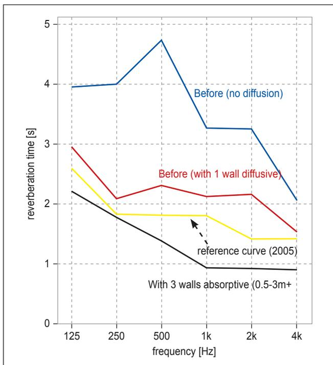
Figure 3. Required and measured reverberation times ( $T_{20}$ ) for 6 octave bands in a large sporthal (38 x 22 x 10) before and after measures.
