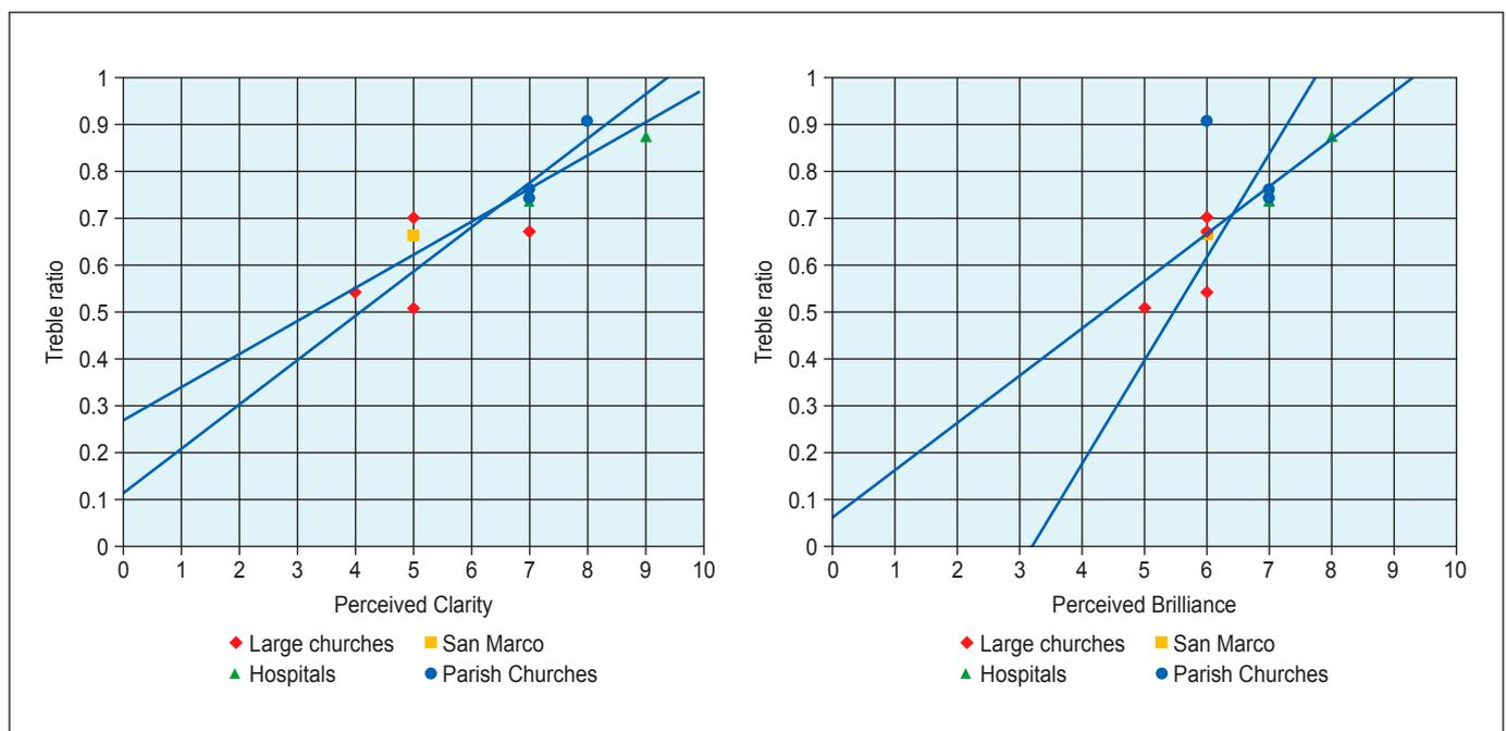
**Figure 14.** (a) The plot of perceived clarity against treble ratio as estimated by the audience. The blue lines are the regression lines of  $y$  against  $x$  and  $x$  against  $y$ . The correlation coefficient is  $r = 0.87$ . (b) The plot of perceived brilliance against treble ratio as estimated by the audience (diamonds). The blue lines are the regression lines of  $y$  against  $x$  and  $x$  against  $y$ . The correlation coefficient is  $r = 0.67$ .
