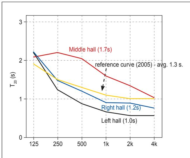
Figure 6. Required and measured reverberation times ( $T_{20}$ ) for 6 octave bands in three 1/3 parts of the sport hall.
