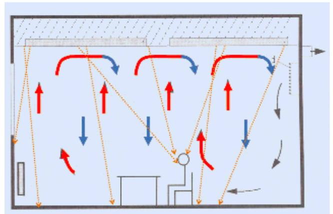
Figure 2. Contribution of thermal mass to summer comfort, through both convection radiation. Regarding convection, warm air (in red) rises and is cooled by contact with the soffit which has been loaded with cold during the night. Cooled air sinks again to the bottom of the room. The dotted lines illustrate radiation.
