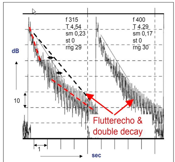
Figure 2. Decay with flutter echoes and double slope for two 1/3 octave bands.
