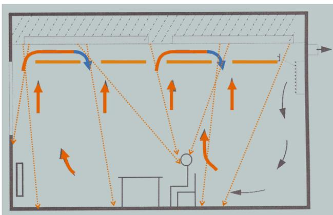
**Figure 5.** Interaction between a discontinuous acoustic ceiling and a room. The horizontal free hanging units should be positioned with enough space between each other, so that they are not an obstacle to convection nor to radiation.
