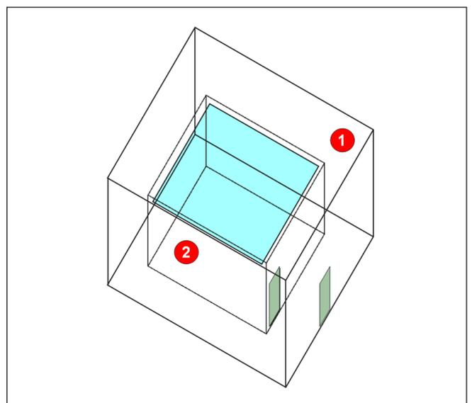
**Figure 6.** Axonometric view of test set-up at SP, Technical Research Institute of Sweden. In blue, the water chilled ceiling.
