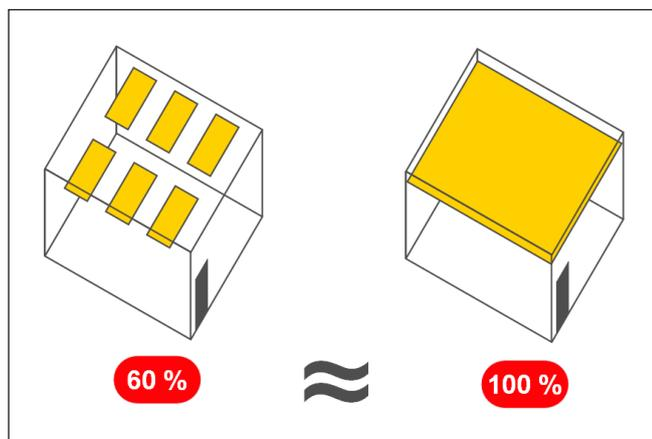
**Figure 9.** Simplified equivalence principle of the contribution of free hanging horizontal acoustic units compared to that of a traditional acoustic ceiling made of the same glass wool material and covering 100 % of the room surface (closed plenum).
