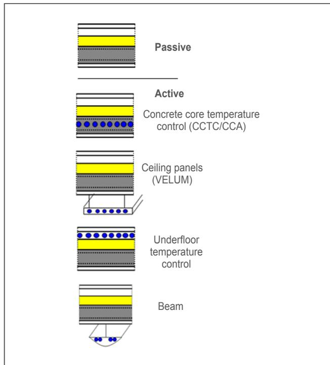
Figure 1. Main concepts using concrete inertia properties. The active form is the combination of the inertia and hydraulic fluid in order to cool down the slabs or bring a thermal comfort using radiation transfer.
