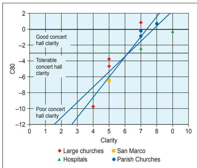
Figure 11. Plot of C80 against perceived clarity. The blue lines are the regression lines of  $y$  against  $x$  and  $x$  against  $y$ . The correlation coefficient is  $r = 0.89$ .
