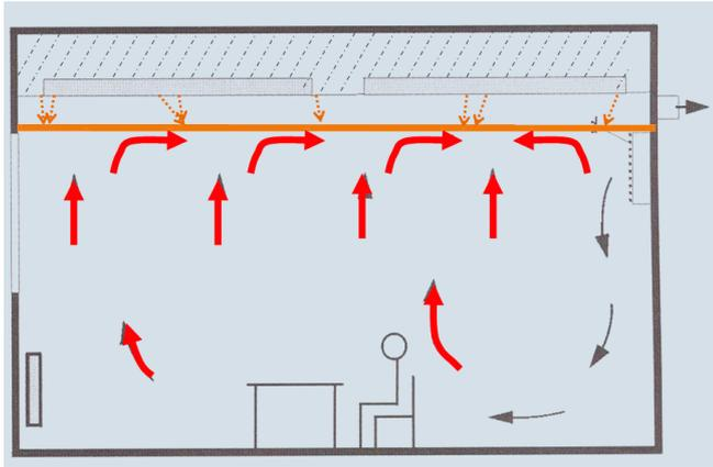
Figure 3. Interaction principle between a full covering acoustic ceiling and thermal exchange in the room. The ceiling is both an obstacle to thermal exchange via radiation and convection.
