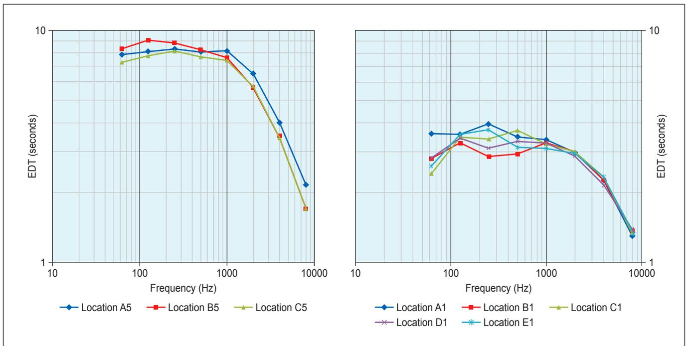
Figure 12. (a) EDT as a function of frequency for listeners in the nave of the Redentore at locations A, B and C. (b) EDT as a function of frequency for listeners in the nave of the San Martino at locations A, B, C, D and E.
