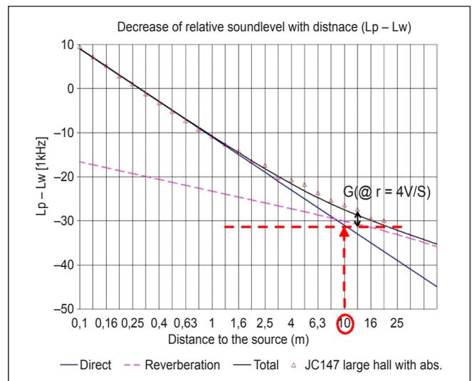
Figure 4. Graph of measured and theoretical decrease of sound level ( $L_p - L_w$ ).
