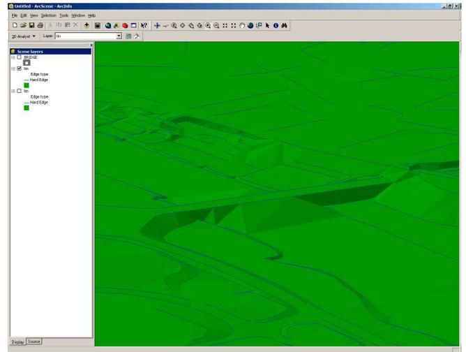
Figure 4. Incorrect interpretation of bridge and terrain over a river.
