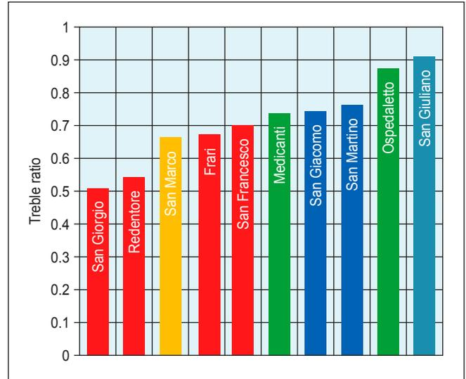
Figure 13. The treble ratio for the 10 churches. The data have been ordered in increasing value of the treble ratio.
