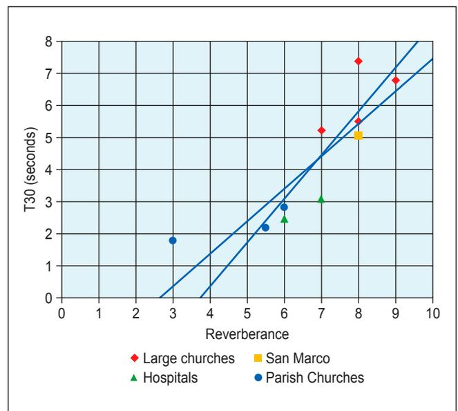
Figure 10. Plot of T30 against average perceived “Reverberance”. The blue lines are the regression lines of y against x and x against y. The correlation coefficient is  $r = 0.87$ .
