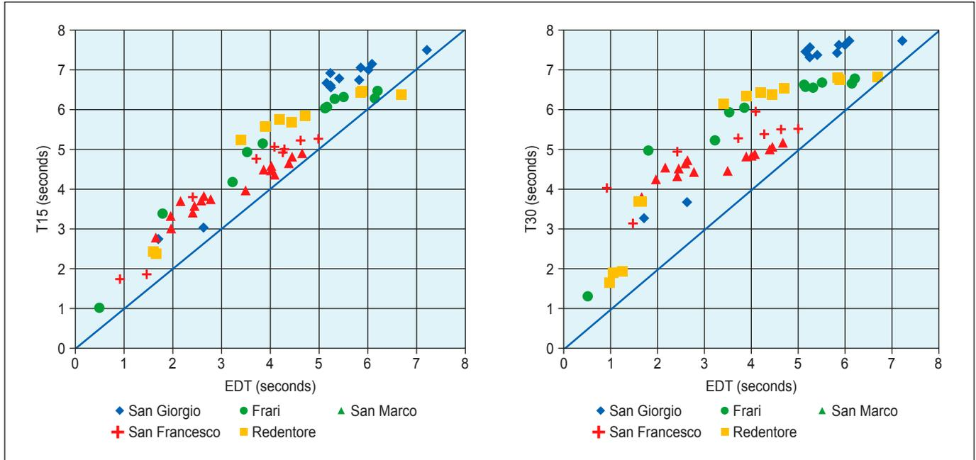
Figure 9. (a) A plot of T15 against EDT for five large churches and all combinations of source and microphone positions for which data were taken. (b) The same plot as (a) for T30 against EDT for the five large churches. In both diagrams, a 45° line is shown.
