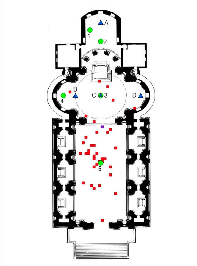
*Figure 1. A plan of the church of the Redentore showing: red squares - positions of audience members; blue triangle - location of acoustic measurement source, identified by letters; green circle - position of acoustic measurement microphone, identified by numbers. The source A and listening positions 1 and 2 are within the friars’ choir.*
