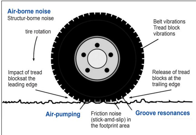
Figure 1. Tyre schematic indicating the main excitation mechanisms upon the interaction of the tyre with the road surface.
