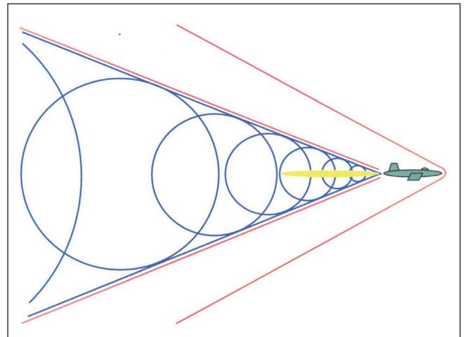
Figure 8. Shock wake of a moving solid body (in red), sound cone of the noise sources (in blue).
