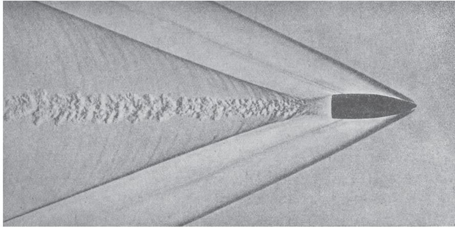
Figure 1. Shock wake and turbulent wake of a rifle bullet. Picture from Ref. [3] (Germany, 1917).
