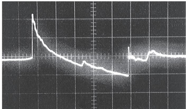
Figure 4. Fighter Dassault Mirage III in flight. Recording of focused sonic boom, from Ref. [15].
