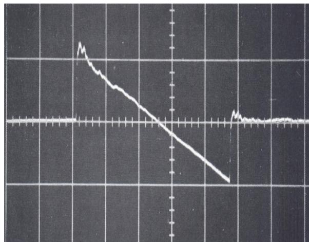
Figure 3. Airliner "Concorde" in flight. Sonic boom recorded at ground level (CEV, Istres, France).
