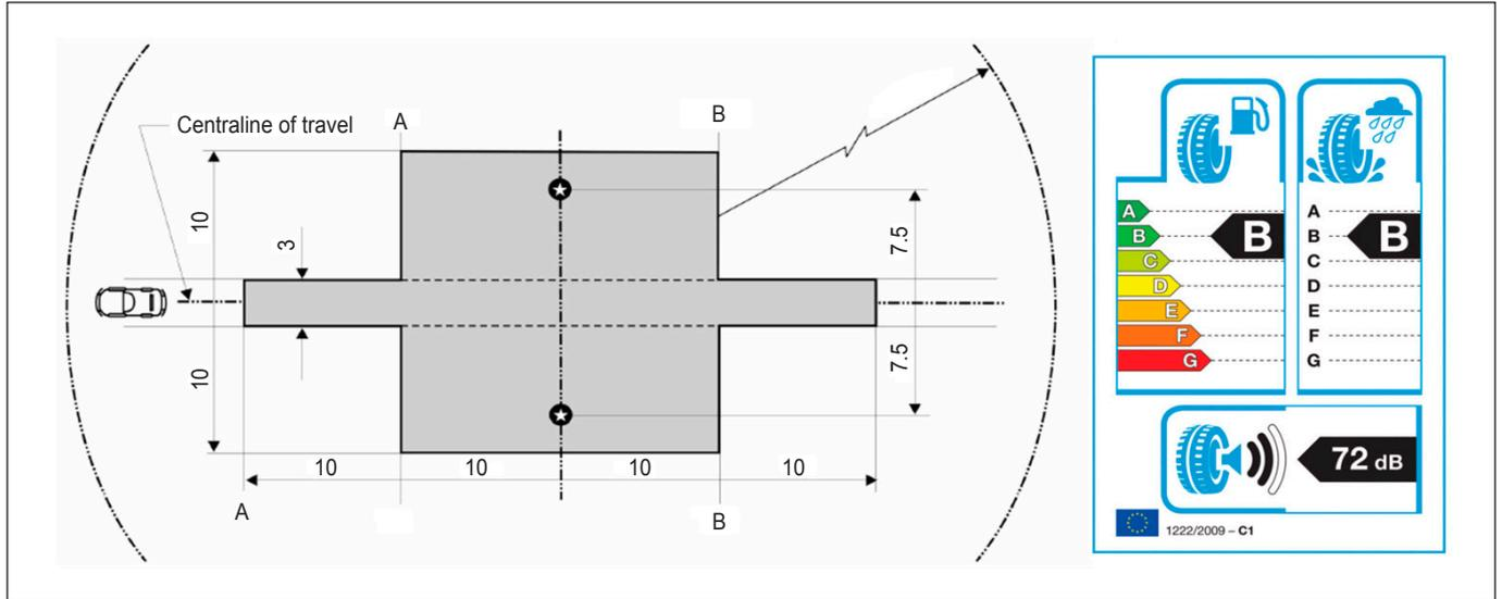
Figure 2. Left: a highly schematic representation of the noise coast-by test [8]. The shaded part represents the test area that is passed by the test vehicle. Two microphones are mounted, each (7.5 ± 0.05) m away from the reference line (centre line of the test track) and (1.2 ± 0.02) m above the ground. Source: Directive 2001/43/EC [10]. Right: example of a label for a C1 class tyre. Source: Reg. 122/2009 [2].
