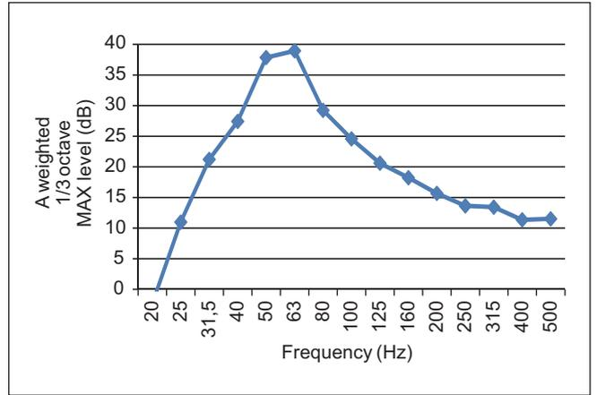
Figure 4. House 1-1, measured groundborne noise.
