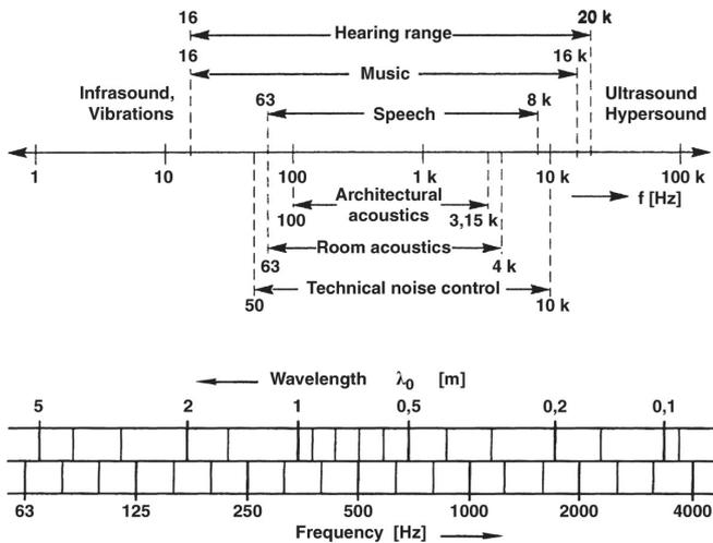
Figure 1. Relevant frequency ranges for practical acoustic tasks (top) and corresponding wavelengths (bottom) after [1].
