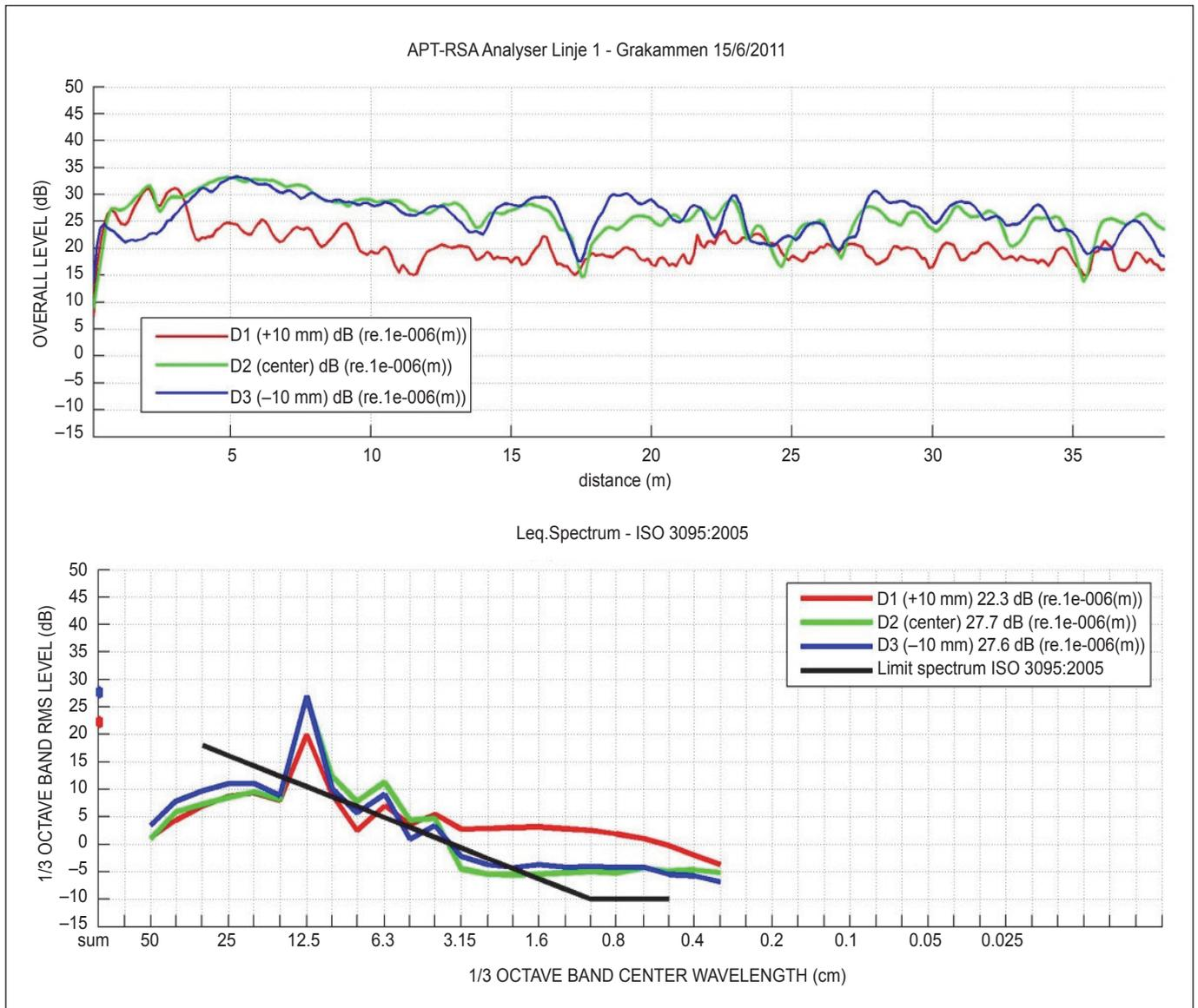
Figure 10. Rail surface analysis for house 1-2 and 1-3.
