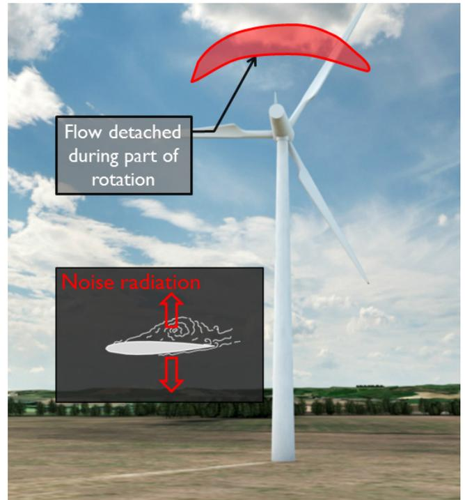
Figure 2. Illustration of detached flow over part of the rotation (partial stall).
