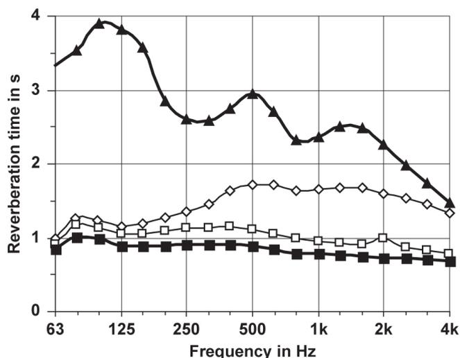
Figure 17. Reverberation times in two similar classrooms without ( $\blacktriangle$ ), respectively with edge absorbers according to Fig. 16; unoccupied ( $\diamond$ ), estimated with 25 users ( $\square$ ), and with additional working utensils ( $\blacksquare$ )
