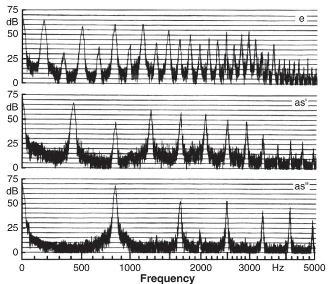
Figure 3. Mean sound spectra when blowing  $E_3, A_4, A_5$  (from top to bottom) on a clarinet after [3].
