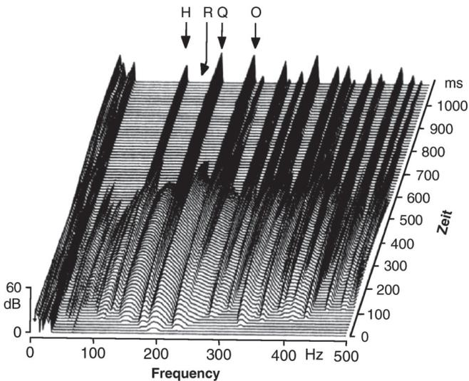
Figure 5. Time evolution of a timpani spectrum of pitch A after [3]; P Principal mode, R 1<sup>st</sup> Ring mode, F Fifth, O Octave.
