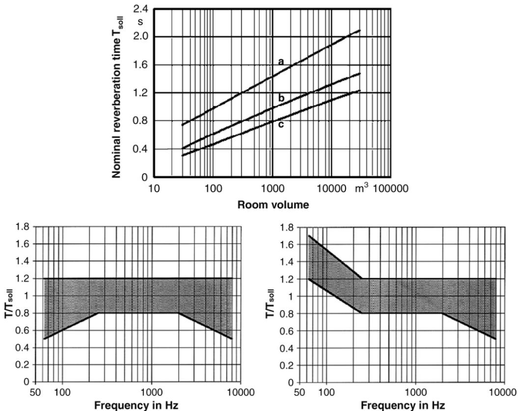
Figure 13. Recommended mean reverberation time  $T_{soll}$  (averaged between 500 Hz and 1000 Hz) in occupied rooms; for musical presentation (a), speech presentation (b), communication and teaching (c) as a function of room volume  $V$  (top) and tolerance range  $T/T_{soll}$  as a function of frequency for speech (bottom left) and music (right) according to DIN 18041-2004.
