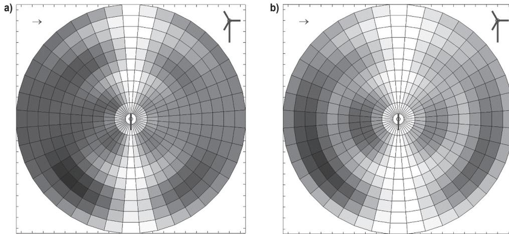
**Figure 3.** Sample instantaneous noise footprints calculated for moderate wind shear (aerial view, wind blowing from left to right) – white corresponds to low noise levels, and black to louder levels, and variations illustrate the presence of modulation, which is mainly present cross-wind in a) (attached flow) and up/down-wind for b) (partially detached flow). From Oerlemans (2011).
