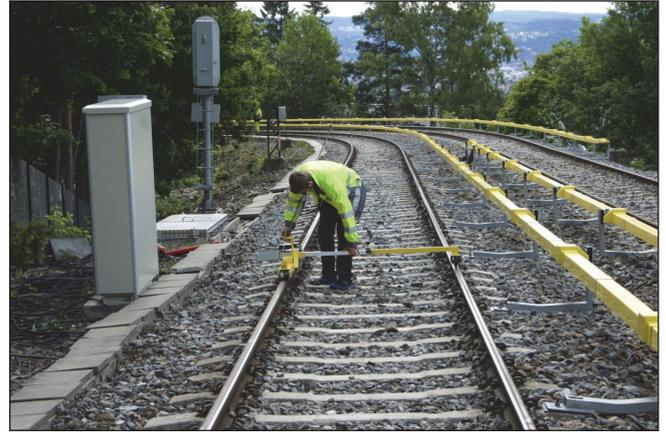
Figure 2. Preparing to measure rail corrugation.
