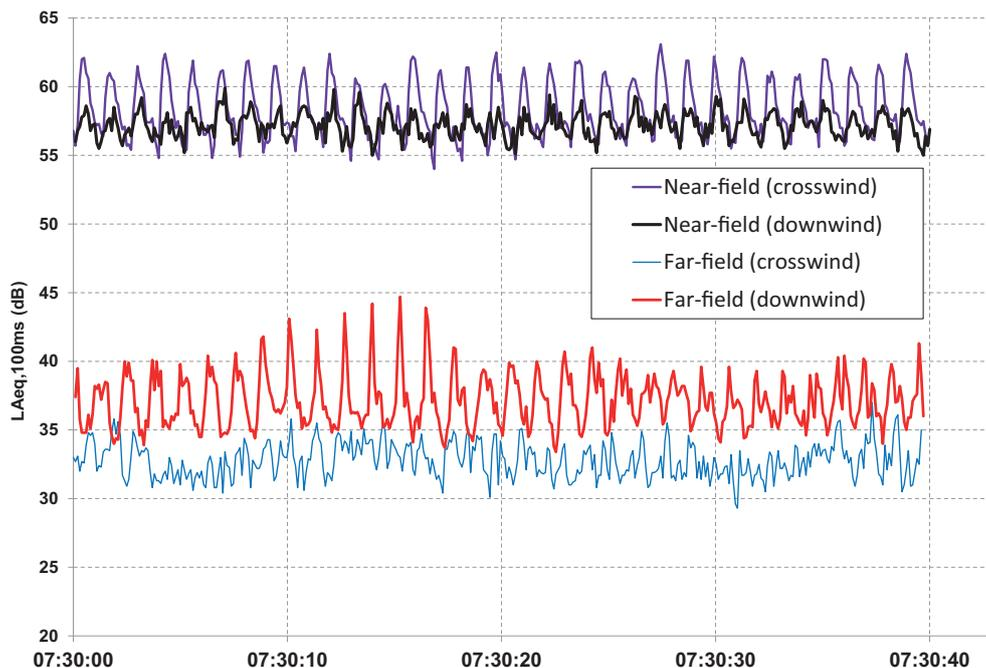
**Figure 4.** Simultaneous time history of measured  $L_{Aeq,100ms}$  levels for a sample OAM period showing: two far-field (downwind and cross-wind) and two near-field locations (cross- and down-wind).
