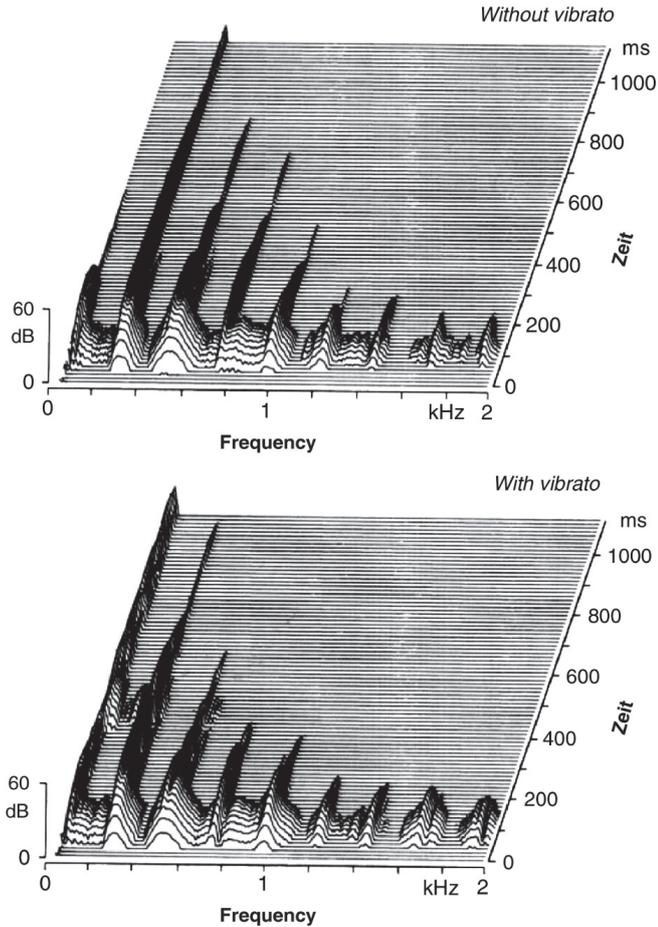
Figure 4. Evolution of the sound spectrum when plucking  $B_3$  on a violin without (top), resp. with vibrato (bottom) after [3].
