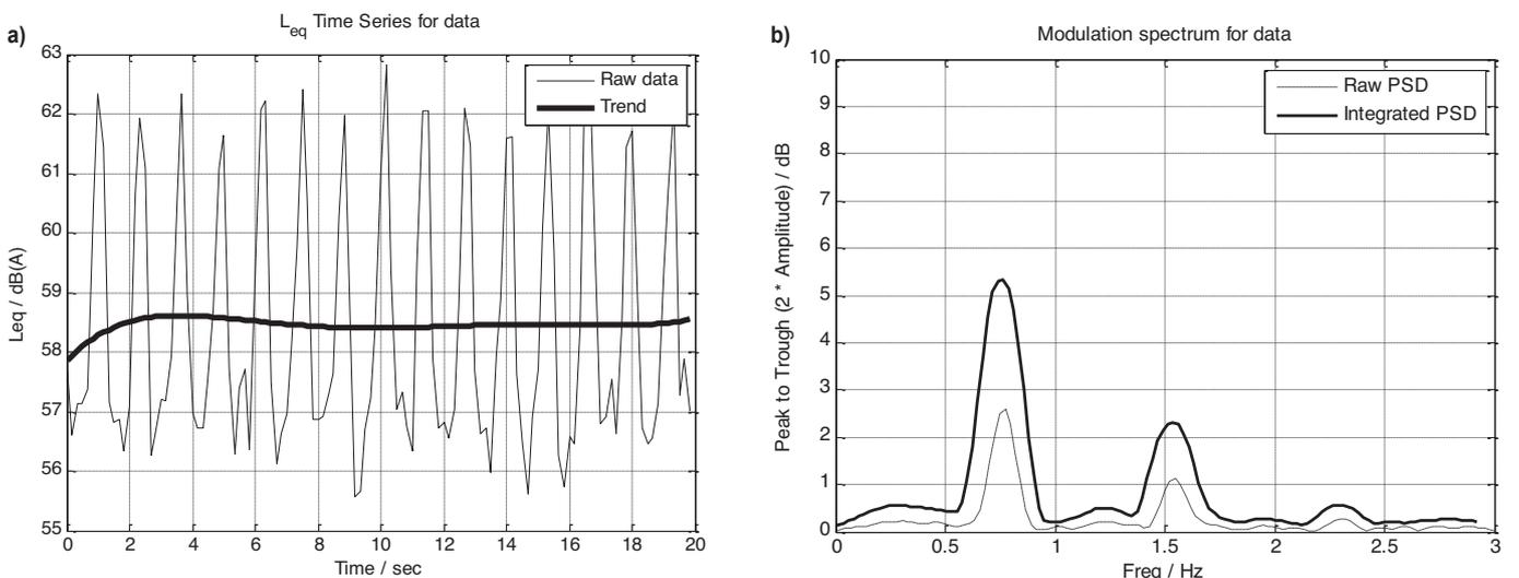
Figure 5. a) Time history ( $L_{Aeq,100ms}$ , arbitrary scale, as a function of time) and b) resulting modulation spectra (as a function of modulation frequency), both raw and integrated, for an artificial AM signal. The peak at the modulation frequency of 0.8Hz is clearly visible in b).
