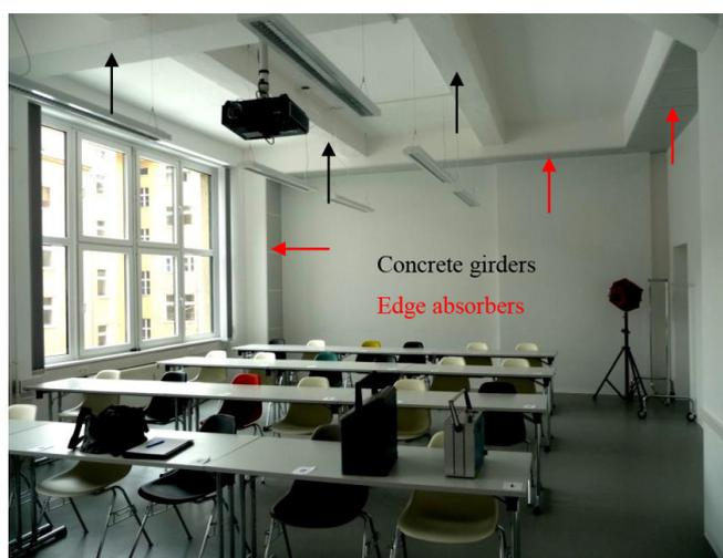
Figure 16. Acoustic retrofitting of a classroom at the University of Media and Communication in Berlin-Kreuzberg with vertical and horizontal edge absorbers [13, 14]
