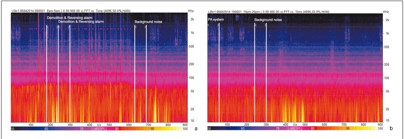
**Figure 2.** Spectra vs. time of two sound recordings (a) and (b). Each figure presents 15 min in duration of a recording, in which the 1-min recording segments are at the indicated areas between the two vertical white lines.
